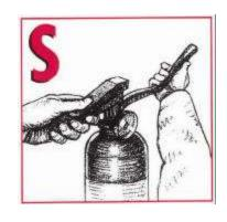
Sweep the extinguisher from side to side covering the area of the fire.
